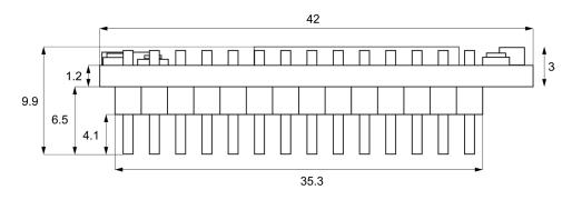
Figure 6 – Mechanical drawing (side view) – Units: mm
