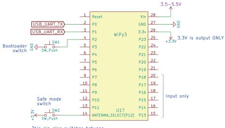
This pin also switches between the on-board antenna and the U.FL connector. For this reason it is not recommended for normal use.
