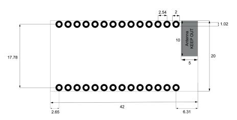
Figure 7 – Recommended land pattern (through hole) – Units: mm
