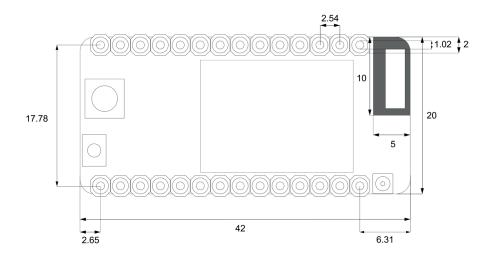
Figure 5 – Mechanical drawing (top down view) – Units: mm
