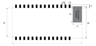
Figure 8 – Recommended land pattern (surface mount) – Units: mm
