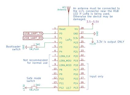
Figure 4 – Minimum required circuit
