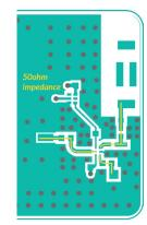
Figure 7 – 50-ohm impedance antenna connections
