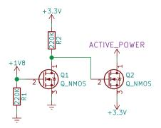
Figure 8 – Power switch for deep sleep mode
